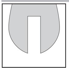
An initial centre hole can be predrilled.
