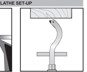
Always use the tool with the straight part of the shaft on the tool rest.
