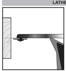
With the tool rest set on centre, place the flat underside of the Hollowmaster on the rest.
