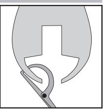
Stop and check the wall thickness at regular intervals.
