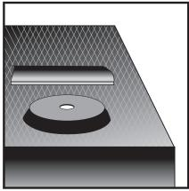
Both tips can be sharpened using a flat sharpening stone or a diamond file (ref RS224). For the perfect sharp edge use the cutter holder (ref 472) in conjunction with the Robert Sorby ProEdge (472 is not suitable for Midi Hollowmaster ref RS130KT).
