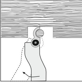
Remove the screw and cutter. Turn the tool over and replace the cutter so that it is facing to the right. Now repeat the previous 2 operations from the left side.
