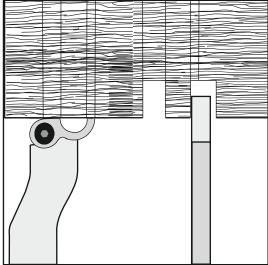
Adjust the cutter back as above and mark on the wood, where the ring will be formed and then remove the waste either side of the lines using a parting tool.
