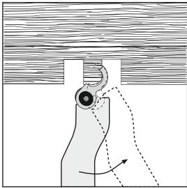
Now move the cutter as above and with just the fluted cutting edge cutting, gently sweep the tool so that the right hand side of the ring can be formed.
