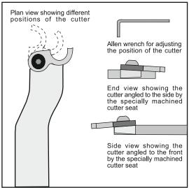
Included with the tool is one captive ring cutter, a machine screw and an allen key / wrench.
