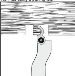
Adjust the cutter so that it is parallel with the shaft and finish the right hand side of the ring.
