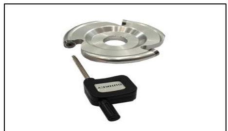
Image 2. Carbide teeth installed on the wheel
