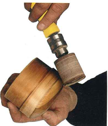
Kirjes Flexible Shaft with a mounted sanding sleeve on a Kirjes Inflatable Sander mod.140.
