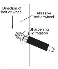
The cutter sharpening jig can be used in two diffferent ways.
