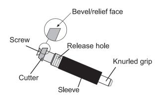
The Robert Sorby cutter sharpening jig is a simple but very effective system for producing a sharp cutting edge on all full round cutters.
